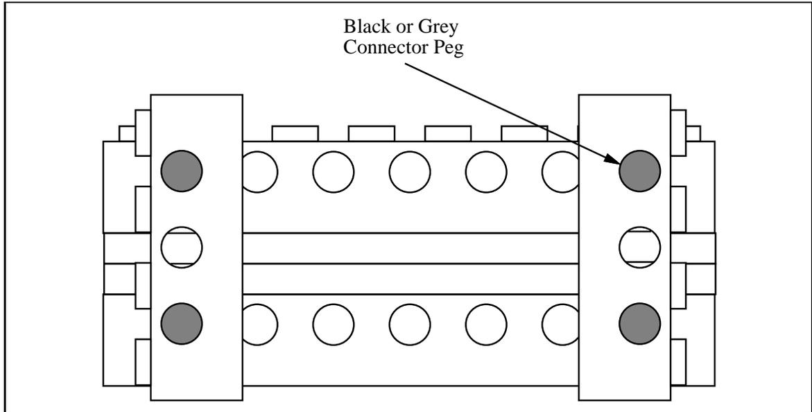
Figure 4.3: Clamping Two Beams at Perfect Vertical Spacing
