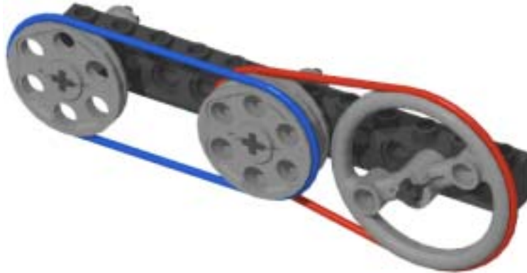
Figure 2-28. Pulleys and Belts
