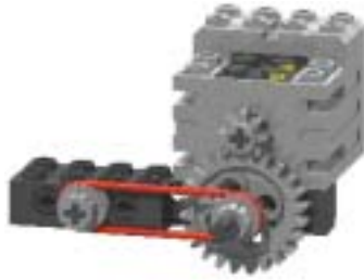
Figure 4-6. Using a Pulley to Increase Drag
