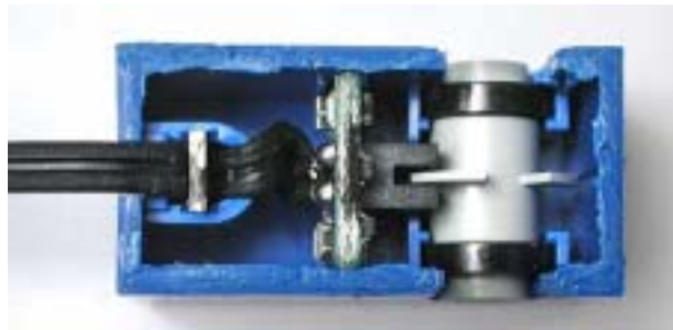
Figure 4-27. Rotation Sensor Internals. DON'T DO THIS!!!
