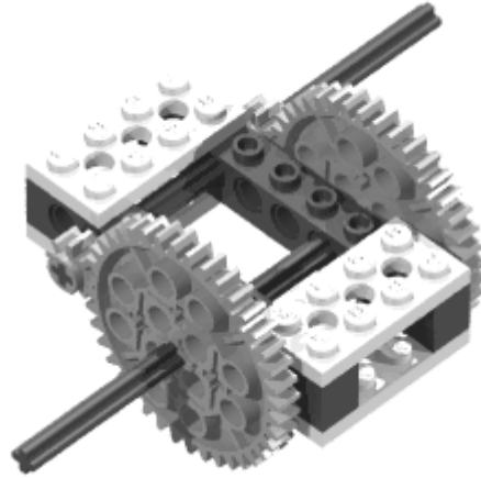
Figure 2-36. Split gear made from LEGO
