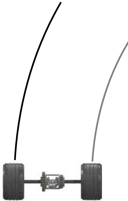
Figure 2-23. During Turns the Wheels Cover Different Distances
