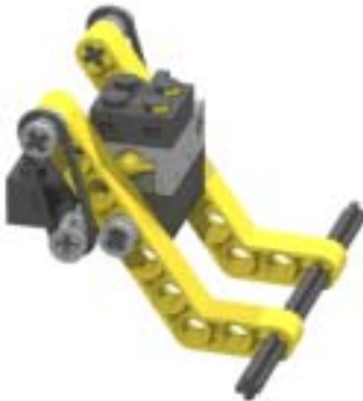
Figure 4-14. Improved Normally Open Bumper
