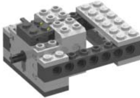
Figure 4-9. Motor Mount Using Rails
