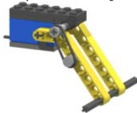
Figure 4-12. A Bumper that Uses the Rotation Sensor
